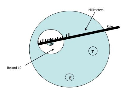
**Figure 6-2:** Measuring the Zone of Inhibition
